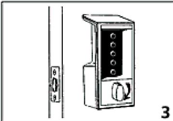
1. Turn the thumbturn to the left (counterclockwise) to the stop position and release. This will clear any random entries from the mechanism.
